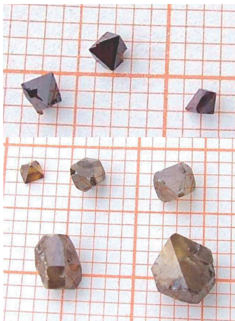
Figure 29. Photograph of prismatic crystals of \text{PbYb}_{0.5}\text{Nb}_{0.5}\text{O}_3 (top) and \text{PbMg}_{0.5}\text{W}_{0.5}\text{O}_3 (bottom) grown out of a \text{PbO-PbF}_2\text{-B}_2\text{O}_3 flux. Reprinted with permission from Ref. [136] Copyright 2008, Elsevier.
